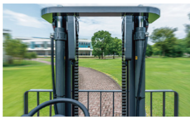
Wide-view mast improves safety in stacking operations.
